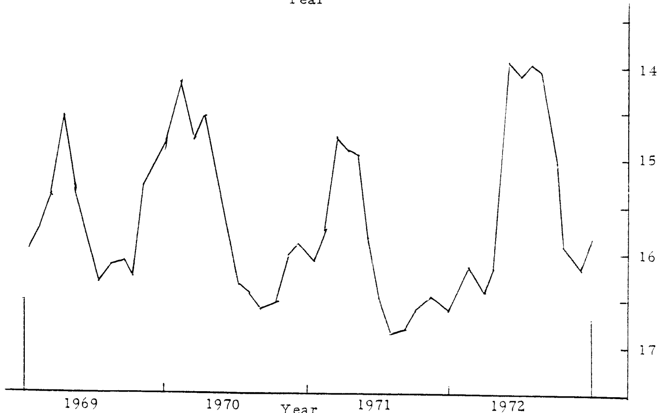
Figure IX (part 1): Graph of water table level below land surface datum from records collected at #2 well, Cochituate State Park, Wayland, Massachusetts.
